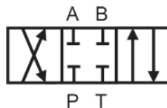
Figure 1: 4 connections / 3 positions DCV
